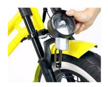
Put the headlight in and fix the front fender and headlight together with screws
