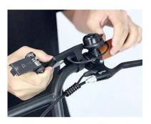
Insert the meter cable in the opposite direction of the arrow
