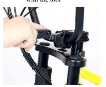
Remove the handlebar screws with tools
