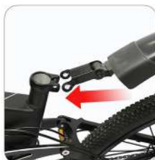
Put the rear fender into the installation position
