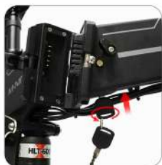
Push the key upwards first, and then turn the key in the direction of the arrow
