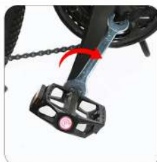
Tighten the right pedal "R" clockwise
