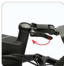
Lock the quick release lever according to the direction
