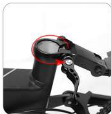
Loosen the quick release lever according to the direction
