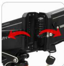
Follow the direction to open the vehicle fold
