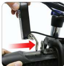
Put the front mudguard and headlight into the front fork position
