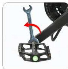
Tighten the left pedal "L" counterclockwise
