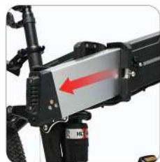
After pulling out the key, take out the battery in the direction of the arrow
