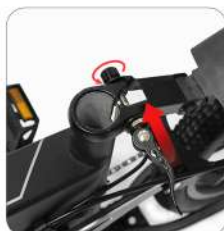
Put in the quick release lever and tighten the quick release lever according to the direction
