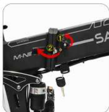
Open the lock in sequence in the direction of the arrow
