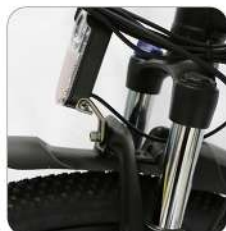
Complete the installation of the headlights and front mudguard
