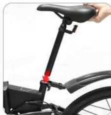
Insert the seat tube in the direction
