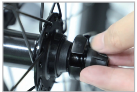
Both sides must be tightened
