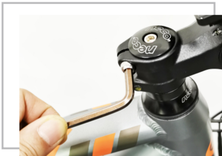
Screw on and tighten
