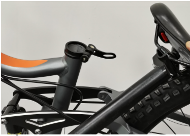
Open the clamp and put the stem into the tube
