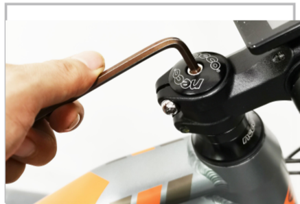
Screw on and tighten
