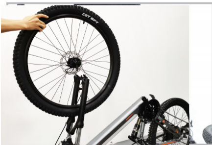
Install the front wheel into the fork
