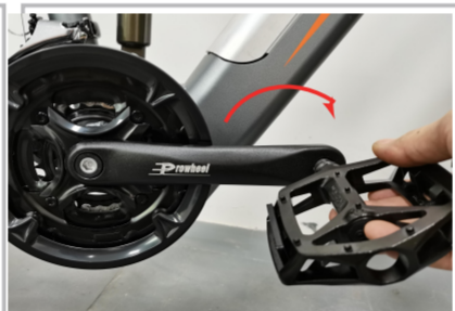
Installed on the chainwheel side crank
