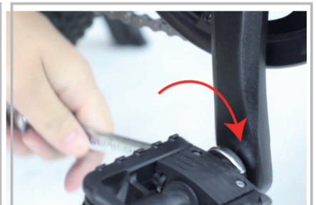
Rotate clockwise to tighten
