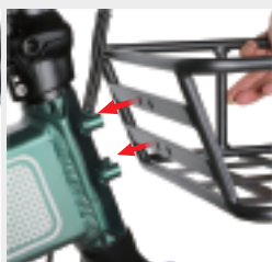
Align the shopping basket with the screw hole and insert the screw
