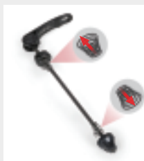
Take out the quick-release clamp, pls pay attention to the direction of spring.
