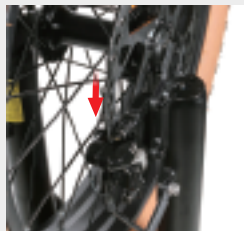
Place the caliper in the disc brake
