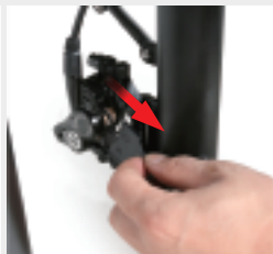
Remove the disc brake gasket
